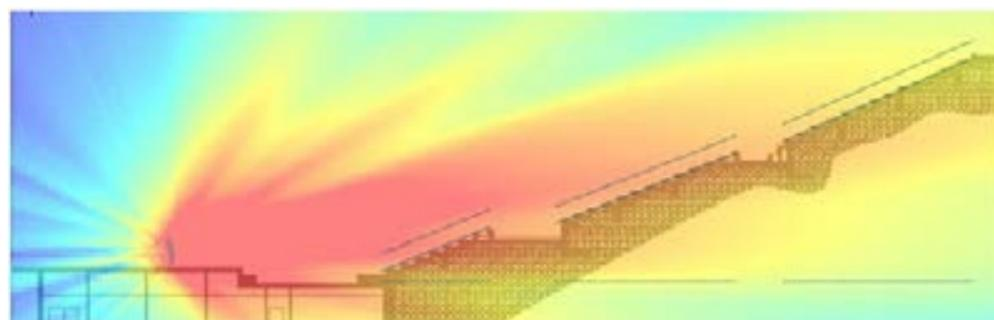
Electronic Beam Steering bypassed
