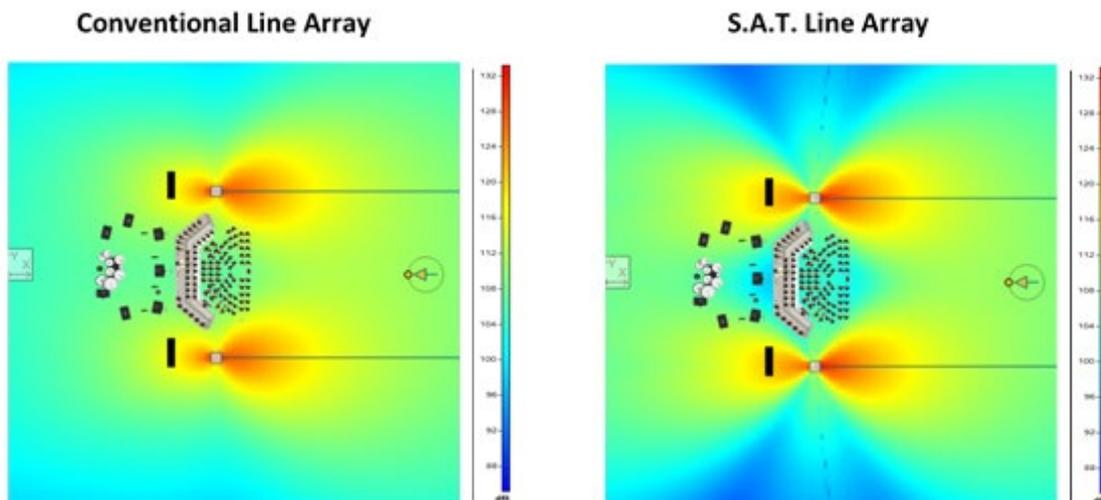
Comparison of the energy distribution of a traditional PA system and a SAT system consisting of 6 KH8 units per side. The simulation shows the SPL values in a third octave band centered at 200 Hz.
