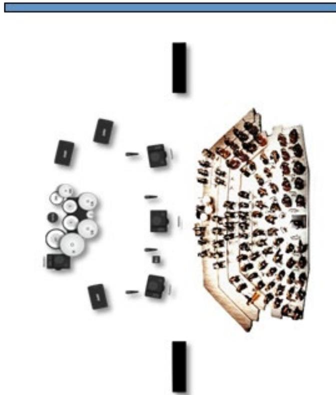
Typical configuration of a live event in which a stereo PA system is mounted
